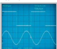
Two asynchronous signals triggered by alternate triggering
